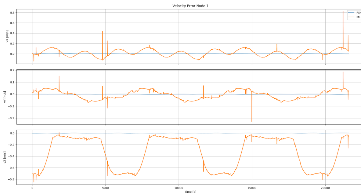
Figure 14: Evolution of velocity error of Runge-Kutta baseline propagator and ML-based propagator.
