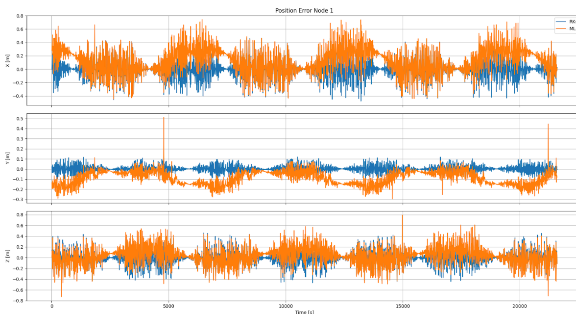
Figure 13: Evolution of position error of Runge-Kutta baseline propagator and ML-based propagator.
